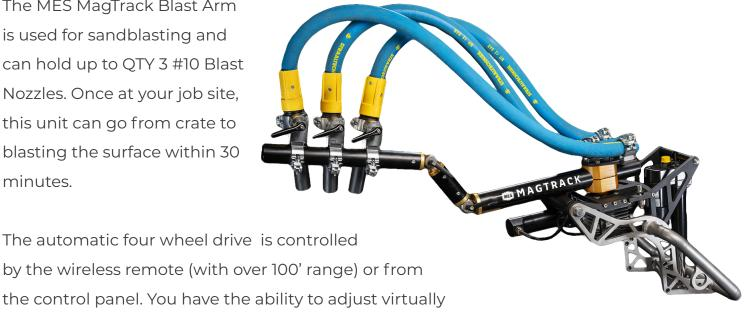
the control panel. You have the ability to adjust virtually any part of this robot at your fingertips. Adjust the swing speed, drive speed, automation speed, and step size all with a few clicks.
